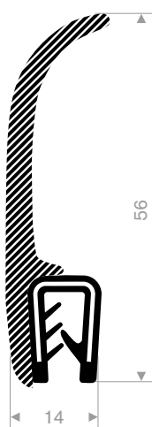
245.00.876 pvc + Sponge rubber clamping range 1-3 mm roll length 25 meter
